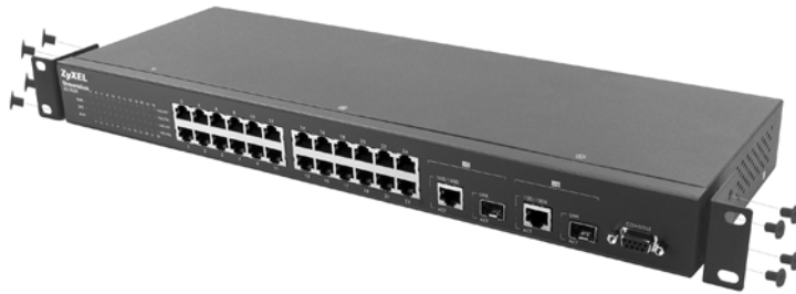
Figure 2-2 Attaching Mounting Brackets and Screws
