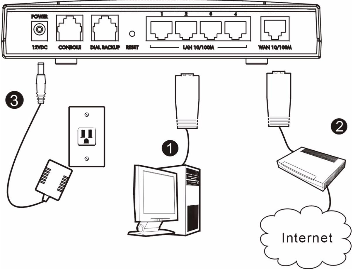
1 Use an Ethernet cable to connect a **LAN** port to a computer.
