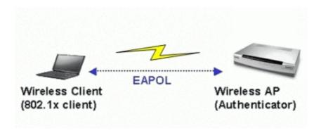
The EAP protocol can support multiple authentication mechanisms, such as MD5-challenge, One-Time Passwords, Generic Token Card, TLS and TTLS etc. Typically, the authenticator will send an initial Identity Request followed by one or more Requests for authentication information. When supplicant receive the EAP request, it will reply associated EAP response. So far, ZyXEL Wireless AP only supports MD-5 challenge authentication mechanism, but will support TLS and TTLS in the future.
