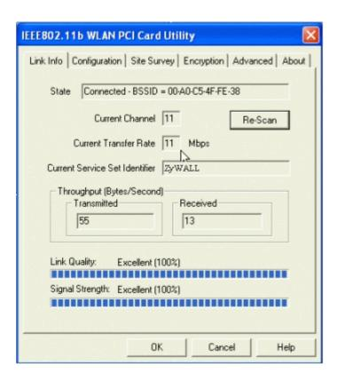
4. It's always a good idea to start with putting the access point at the corner of the room and walk away from the access point in a systematic manner. Record down the changes at point where transfer rate drop and the link quality and signal strength information on the diagram as you go alone.
