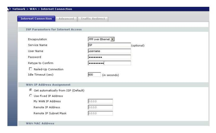
Select "Get automatically from ISP" if the ISP provides the IP dynamically, otherwise select "Use Fixed IP address" and enter the static IP given by ISP in the box following "MY WAN IP Address" field.
