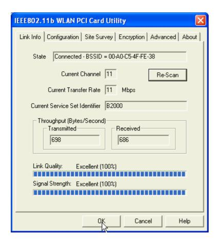
6. After the client have associated with the selected AP. The linked AP's channel, current linkup rate, SSID, link quality, and signal strength will show on the Link Info page. You now successfully associate with the selected AP with Infrastructure Mode.
