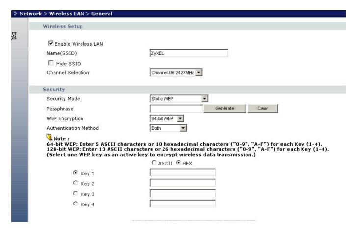
b. Configure the desired configuration on P320W. For each configurable parameter, what it is and how it function, please refer to the user's guide for detail or web help located on the page.
