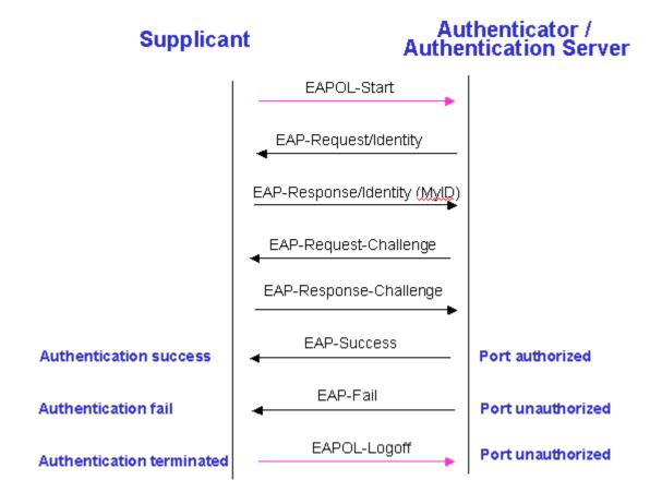
The EAPOL packet contains the following fields: protocol version, packet type, packet body length and packet body. Most of the fields are obvious. The packet type can have four different values, and these values are described below:
