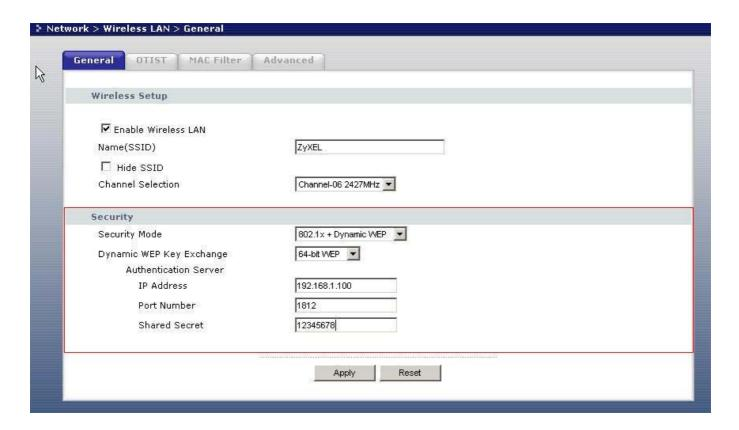
After 802.1x authentication function is enabled, you have to setup the authentication server, you need to specify the location and port of an <u>external RADIUS authentication server</u>.
