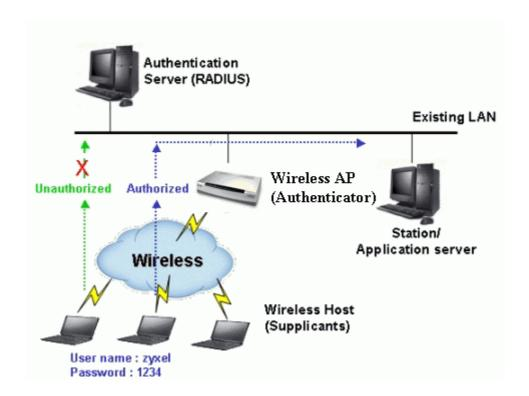
IEEE 802.1x authentication is a client-server architecture delivered with EAPOL (Extensible Authentication Protocol over LAN). The authentication server authenticates each client connected to a Access Point (For Wireless LAN) or switch port (for Ethernet) before accessing any services offered by the Wireless AP. 802.1x contains tree major components:
