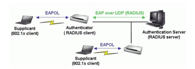
When the client supplies its identity, the authenticator begins its role as the intermediary, passing EAP frames between the supplicant and the authentication server until authentication succeeds or fails. If the authentication succeeds, the switch port becomes authorized. The specific exchange of EAP frames depends on the authentication method being used. The figure below shows a message exchange initiated by the client using the MD5 Challenge authentication method with a RADIUS server.
