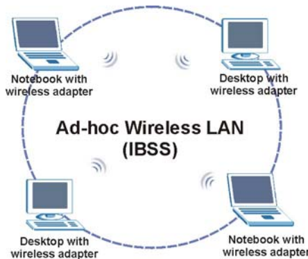
Figure 12-1 IBSS (Ad-hoc) Wireless LAN
