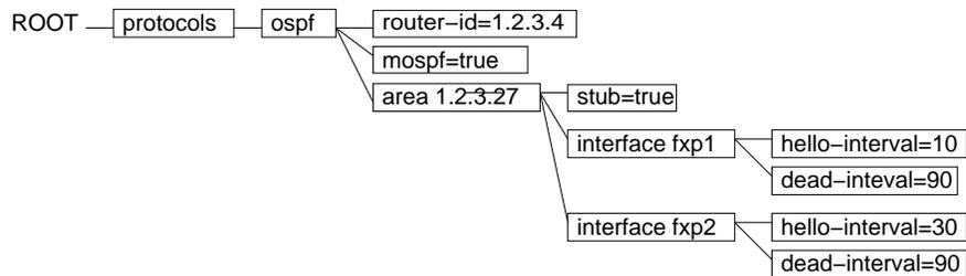
Note that configuration tree nodes have been created for `dead-interval` and (in the case of `fxp1`) for `hello-interval` even though this was not mentioned in the configuration file. This is because the template tree contains a default value for this leaf node. Also, in case of configuring a boolean variable (e.g., of type `bool` or `toggle`) such as `mospf`, typing the variable name itself (e.g., `mospf`) is equivalent to assigning it value of `true` (e.g., `mospf: true`).
