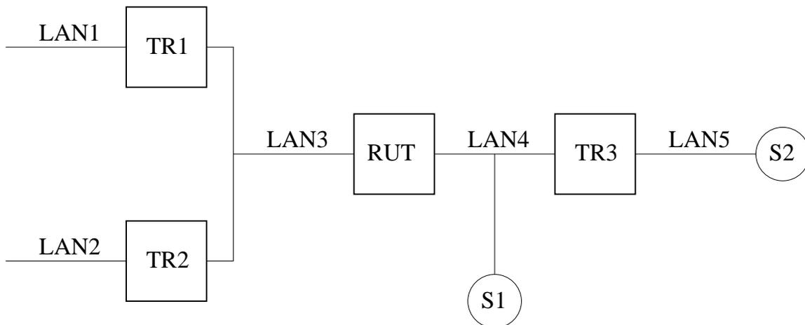
Figure 4.3: Receiving (S,G) Join/Prune messages test setup
