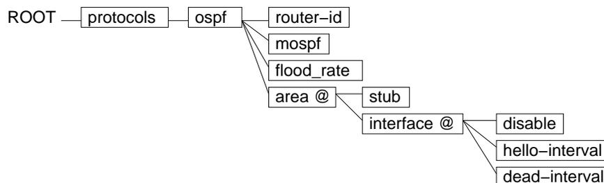
The same node may occur multiple times in the template file. This might happen because the node can take more than one type (for example, it might have an IPv4 or an IPv6 address), or it might happen because the second definition adds information to the existing definition.
