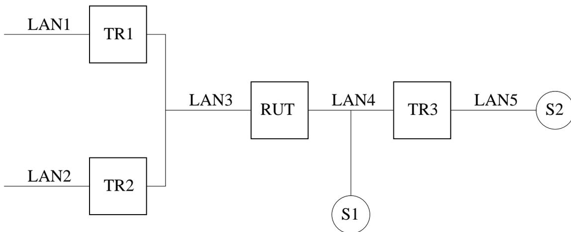
Figure 4.4: Receiving (S,G,rpt) Join/Prune messages test setup
