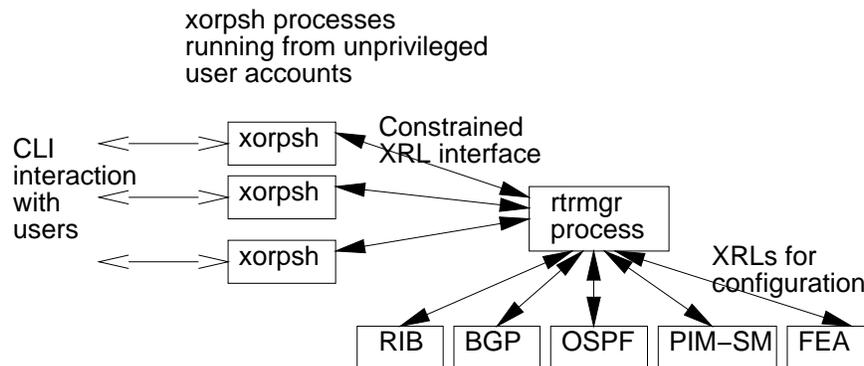
The interface between the `rtmgr` and a `xorpsh` instance consists of XRLs that the `xorpsh` may call to query or configure `rtmgr`, and a few XRLs that the `rtmgr` may asynchronously call to alert the `xorpsh` process to certain events.
