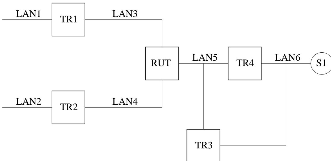
Figure 4.6: Sending (\*,G) Join/Prune Messages test setup
