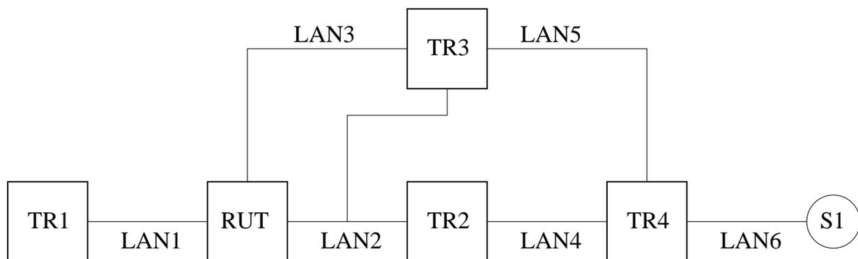
Figure 5.1: (S,G) Assert message state machine test setup
