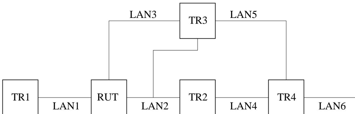
Figure 6.7: Semantic fragmentation of BSMs test setup
