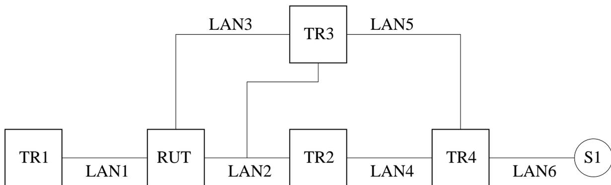
Figure 5.2: (\*,G) Assert message state machine test setup
