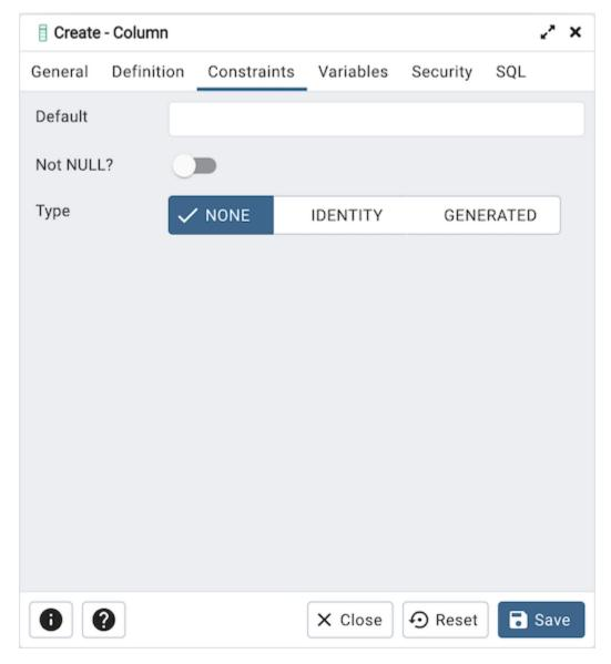
Use the fields in the *Constraints* tab to specify constraints for the column. (Fields are disabled if inapplicable.)
