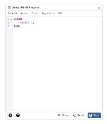
• Use the *Code* field to write the code that executes when the program is invoked. This tab is only enabled when the type of the program is set to 'PLSQL BLOCK'.
