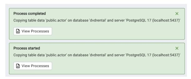
Use the *View Processes* button on the notification to open the *Process Watcher* and review detailed information about the execution of the command that performed the import or export:
