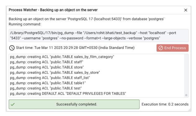
The Process Watcher logs all the activity associated with the process/task and provides additional information for troubleshooting Use the **End Process** button to end the process.
