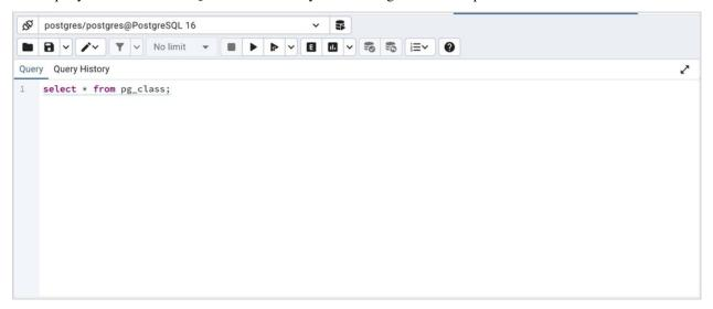
To use autocomplete, begin typing your query; when you would like the Query editor to suggest object names or commands that might be next in your query, press the Control+Space key combination. For example, type "SELECT \* FROM" (without quotes, but with a trailing space), and then press the Control+Space key combination to select from a popup menu of autocomplete options.
