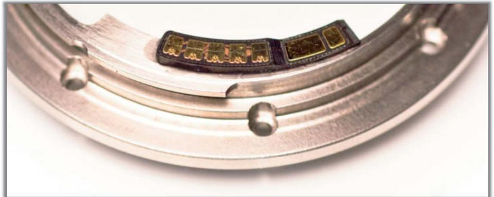
The Dandelion AF confirm chip (above, attached to a Leitax adapter) is programmable, enabling it to transmit camera Exif data and autofocus assist information
