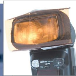
Flash filters are not denoted with numbers like lens filters, but are instead named using abbreviations that indicate their color. For example, a CTO (Color Temperature Orange)
