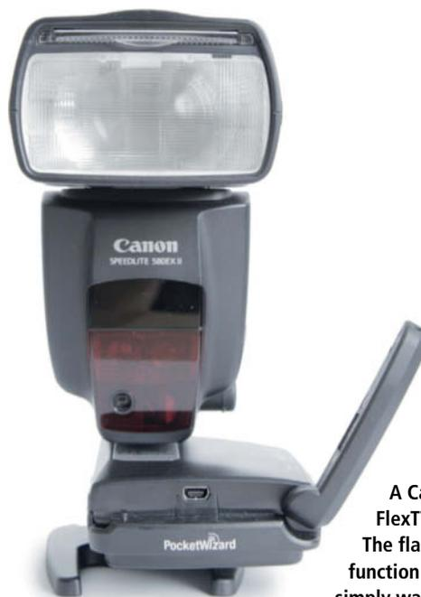
A Canon flash mounted on the PocketWizard FlexTT5 (shown with its antenna extended for use). The flash has to be switched to normal E-TTL mode to function properly – in E-TTL slave mode it would simply wait for infrared signals.
