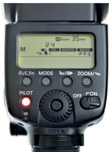
The Canon 580EX II in master mode and set to manual slave control. Slave control is either completely manual or completely via TTL. You can select output individually for up to three groups (A, B and C). The illustration shows group C set to 1/4 power.
