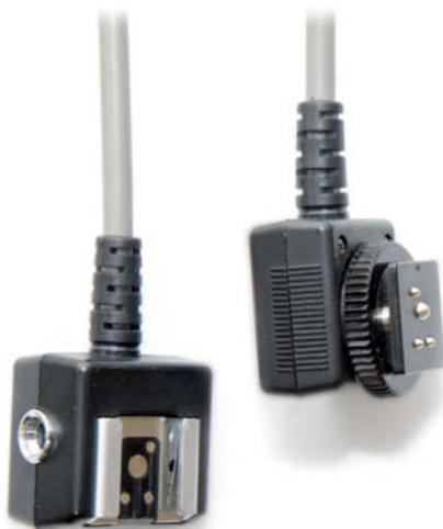
These are the two ends of a Nikon SC-17 TTL remote cord (now superseded by the SC-28). The right-hand end is attached to the camera’s hot shoe and the flash is attached to the other end. The two (proprietary) sockets on the sides of the flash end can be used to attach and control additional Nikon flash units.
