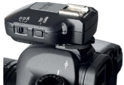
The PocketWizard MiniTT1 transmitter mounted on a Canon camera. In master mode, the unit “speaks” E-TTL with its slaves, but the lack of a user interface makes it impossible to enter flash compensation values or to alter flash output.
