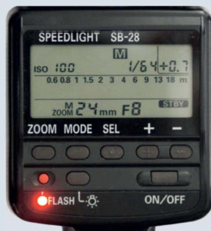
The Nikon SB-28 Speedlight allows you to set flash output in 1/3-stop increments with a minimum of 1/64 power
