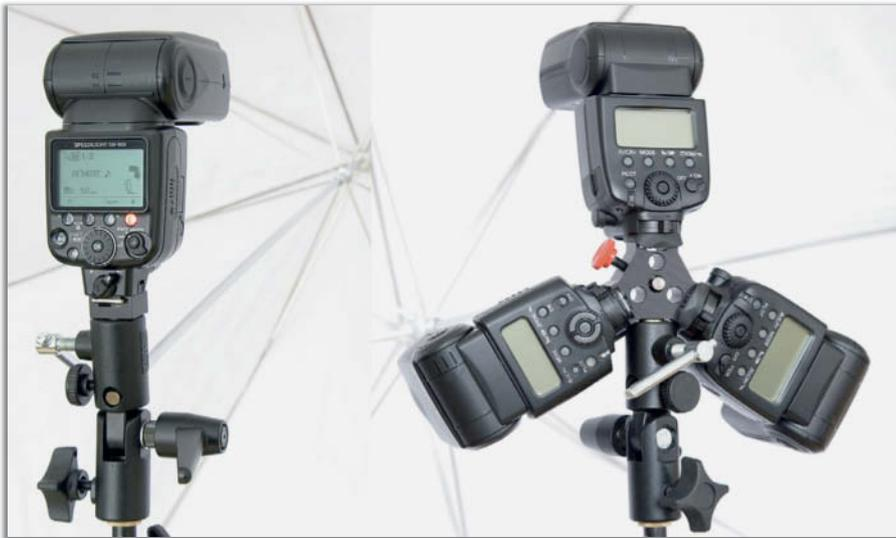
The Manfrotto 026 swivel umbrella adapter (on the left) has differently shaped grips for each adjuster – smart ergonomic thinking! The picture on the right shows the IDC Photography Triple Threat flash bracket with three flashes mounted.
