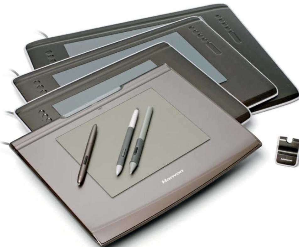
tures of the *Media Tablet*. The mechanical jog wheels have been replaced by recessed sensors with functions that are selected using the four keys located between them. One of these toggles each of the other three between two different states, giving the user a choice of six preset sensor functions.
