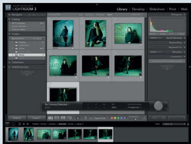
egant solution for a broad selection of Canon, Leica and Nikon cameras. The tethered capture feature allows you to select a Develop preset and a destination folder in a simple dialog window and presents an additional control window that displays aperture, shutter speed, ISO and white balance settings, and which includes a remote shutter-release button. The displayed settings cannot, however, be adjusted via the computer interface.
