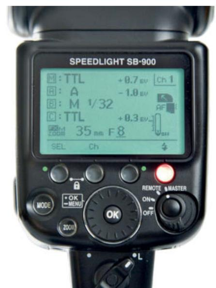
The Nikon SB-900 being used as a master unit. Flash mode, exposure compensation values and manual output settings can be individually set for the master, and all three remote groups using user-friendly backlit buttons – this is as good as accessory flash gets!
