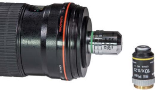
Nikon microscope objectives can be mounted on a host lens using an adaptor with an RMS thread. They enable full-frame captures of up to 40× or 64× using an APS-C camera.
