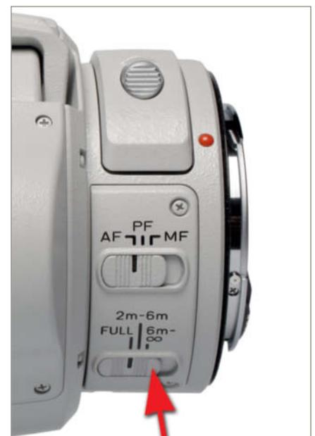
The focusing distance range selector switch limits the focus range to reduce autofocus reaction times and speed up shooting
