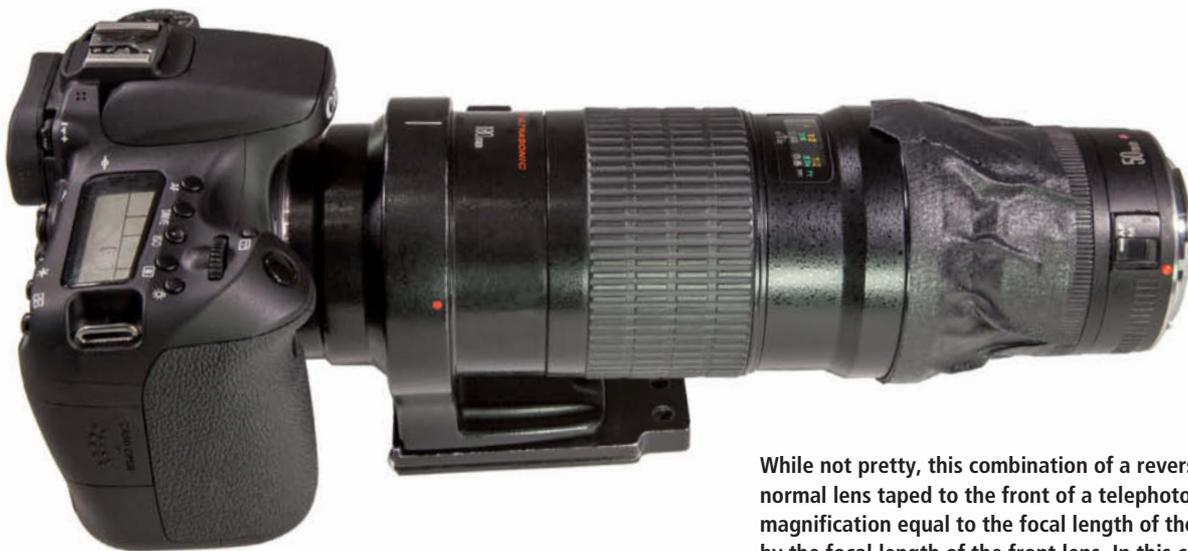
While not pretty, this combination of a reversed normal lens taped to the front of a telephoto achieves a magnification equal to the focal length of the rear lens divided by the focal length of the front lens. In this case, the EOS 70D with its crop factor of 1.6, the 180mm macro and the 50mm lens offer a final magnification of 5.8x.
