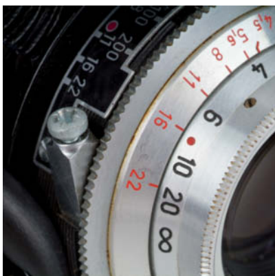
4 Inserting a thin screw into the cable release socket enables you to fix the shutter in its open position
