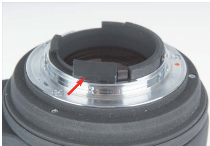
If your lens doesn't have a manually adjustable aperture ring, you will need to deactivate the aperture mechanism yourself. Here, I used a small piece of plastic to wedge it in position.
