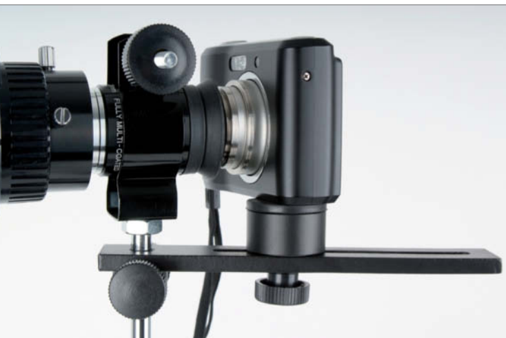
You can use an adapter to attach a compact camera to your home-made telescope
